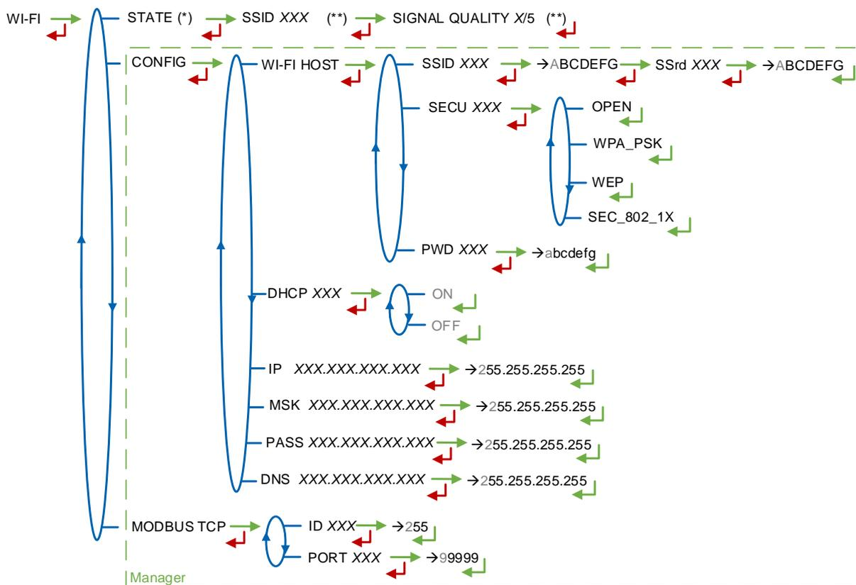
(\*) NOT AVAILABLE (the calculator is not equipped) / DISCONNECTED / CONNECTED
