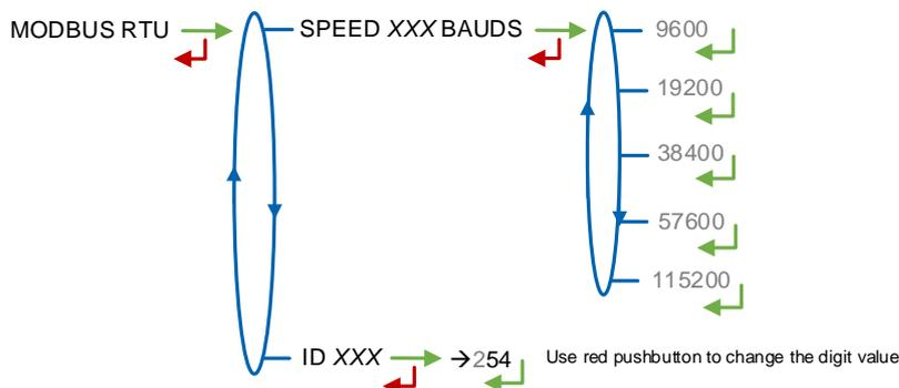
**SPEED:** Speed of the Modbus connection
