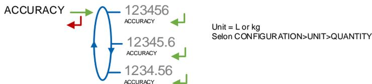
**FLOWRATE:** Choose the accuracy of the quantity that will be displayed and printed. According to the unit set in menu CONFIGURATION>UNIT>QUANTITY (measure of a volume or a mass).
