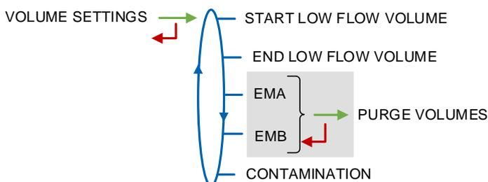
**START LOW FLOW VOLUME or START LOW FLOW MASS:** Volume or mass delivered in low flowrate before switching in high flowrate.
