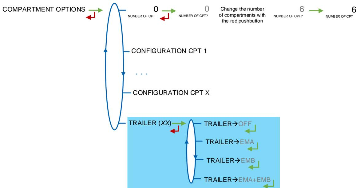
This menu is used to configure the compartments and their assignment to each measuring system, if required. First, set the number of compartments.
