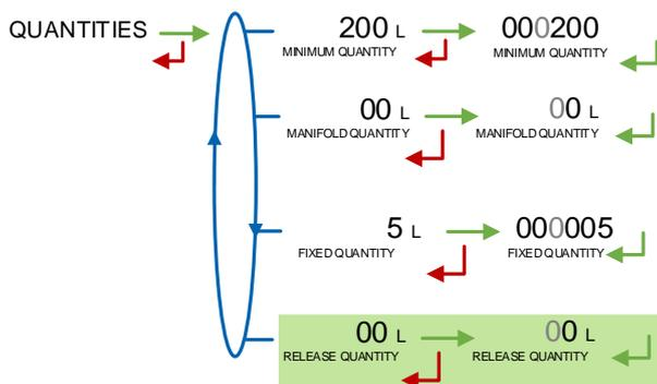
**MINIMUM QUANTITY:** Set the minimum quantity of the EMA measuring system. This value is given by the association of the turbine meter, the MICROCOMPT+ and other parts of the measuring system.
