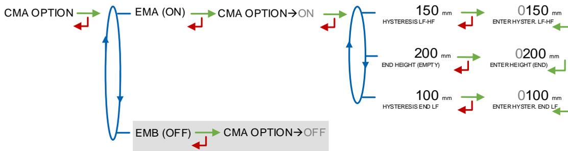
**HYSTERESIS LF-HF:** At the beginning of a measurement or following an intermediate stop. Before switching again from low to high flowrate, the calculator-indicator checks the total between LOW FLOW HEIGHT and HYSTERIS LF-HF.
