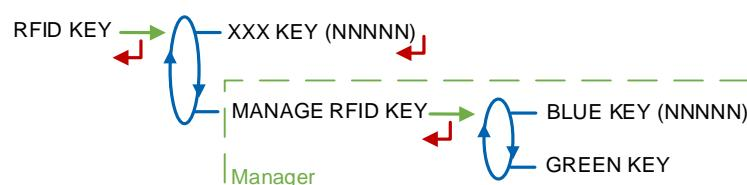
**XXX KEY (NNNNN):** Displays the information about the RFID placed on the screen with: XXX = color and (NNNNN) = identifier. E.g.: RED KEY (01234)
