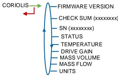
This sub-menu allows to display the states and sizes from the CORIOLIS.
