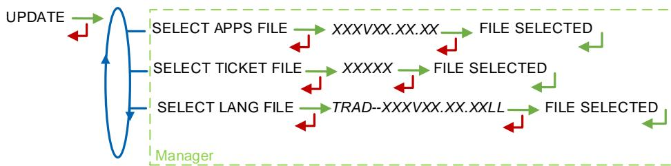
**SELECT APPS FILE (\*)** – Access restricted to the Manager with green key and/or to the Maintenance with red key. Used to display and select the version(s) of the application available on the SD card. NO FILE is displayed if there is no file to download.
