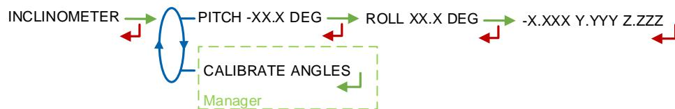
**PITCH:** Used to display the bank angles of the truck and the inclinometer raw data.
