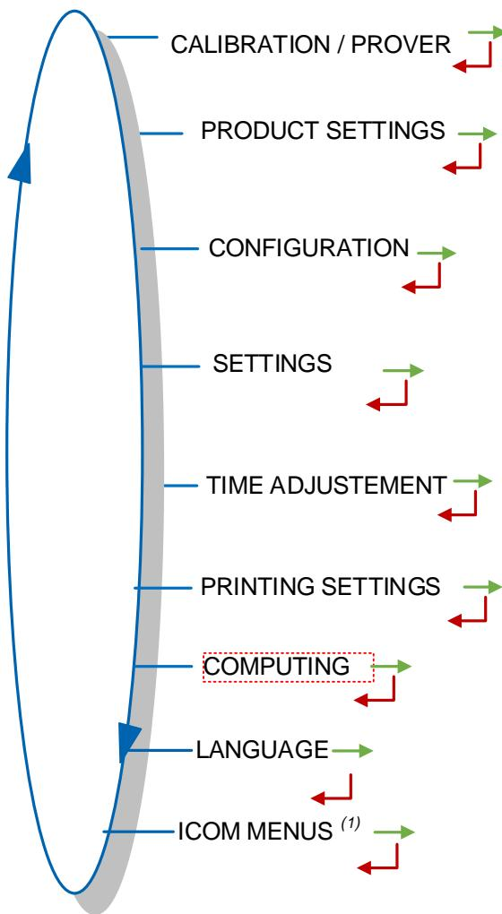
**ICOM MENUS<sup>(1)</sup>:** The submenus differ according to the authorised access level: (Operator level, Manager level, Maintenance level).
