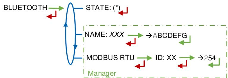
(\*) NOT AVAILABLE (the calculator is not equipped) / DISCONNECTED / CONNECTED
