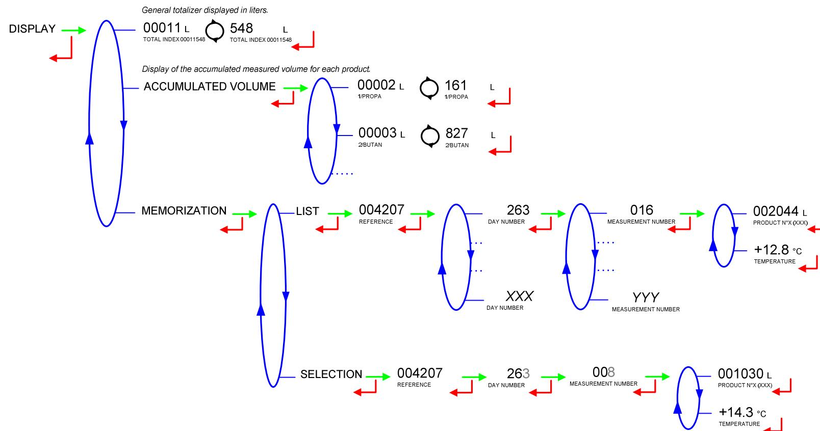
Display sequence of measurement results memorized by LPGTRONIC.
