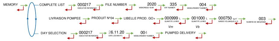
For each measurement, are displayed: the distribution mode (pumped or gravity), the product number and name, the delivered quantity Vm then Vb, the density.
