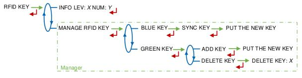
**INFO**: Display of the level and the identifier of the RFID key (blue key: Level1-User, green key: Level2-Manager, red key: Level3-Maintenance)
