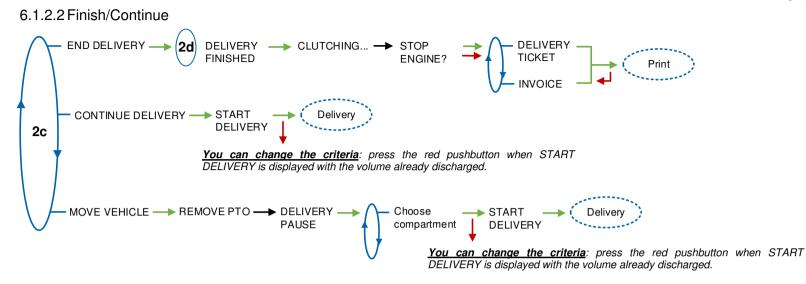
If it's necessary to move the vehicle, the distribution has to be stopped for a moment, then choose the MOVE VEHICLE item. The GRAVITRONIQUE switches off the power take-off, clutches the engine and freezes the MICROCOMPT+ indicator on DELIVERY PAUSE. Press the green OK BUTTON to continue distribution
