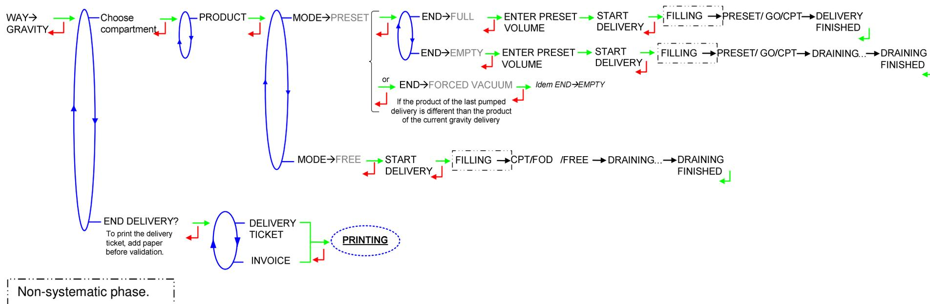
In case of an intentional interruption of delivery with the red STOP BUTTON, the following sequence is proposed:
