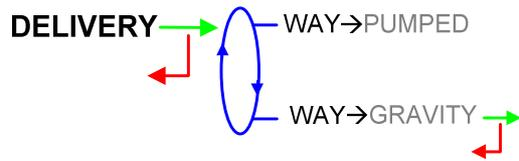
For a preset distribution, the choice is given to end with the manifold full or empty. However if the gravity delivery is made with a product different than the last pumped-delivered product, the GRAVITRONIQUE requires to end with the manifold empty in order to avoid any mixture of product: END→EMPTY must be validated.
