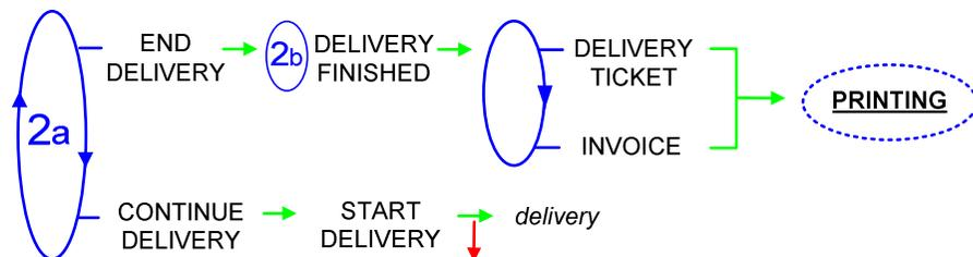
**To change the delivery criteria:** press the red pushbutton when START DELIVERY is displayed with the volume already discharged.
