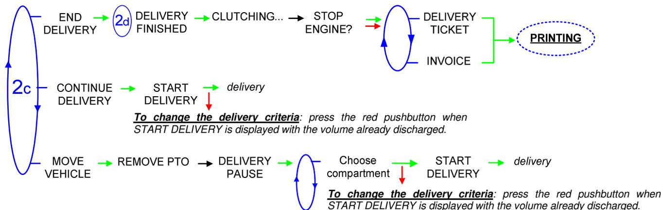
If it's necessary to move the vehicle, the distribution has to be stopped for a moment, then choose the MOVE VEHICLE item. The GRAVITRONIQUE switches off the power take-off, clutches the engine and freezes the MICROCOMPT+ indicator on DELIVERY PAUSE. Press the green OK BUTTON to continue distribution
