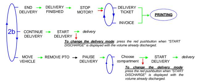
If it's necessary to move the vehicle, the distribution has to be stopped for a moment, then choose the "MOVE VEHICLE" item. The GRAVITRONIQUE switches off the power take-off, clutches the engine and freezes the MICROCOMPT indicator on "PAUSE". Press green button to continue distribution.
