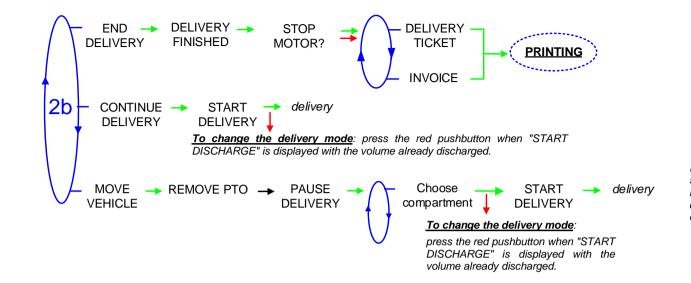
If it's necessary to move the vehicle, the distribution has to be stopped for a moment, then choose the "MOVE VEHICLE" item. The GRAVITRONIQUE switches off the power take-off, clutches the engine and freezes the MICROCOMPT indicator on "PAUSE". Press green button to continue distribution.
