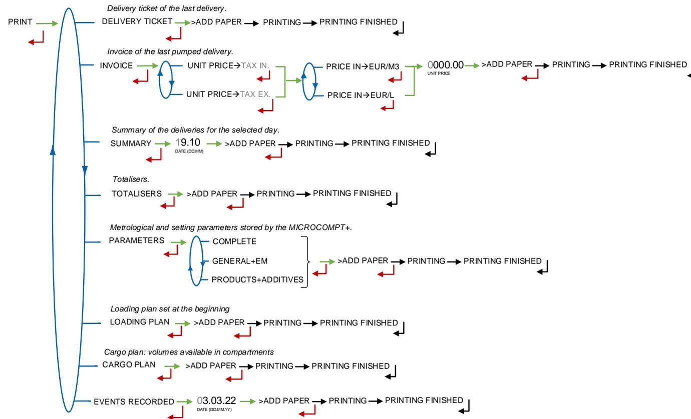
According to the needs, the **PARAMETERS** sub-menu prints all or part of the parameters. Three sub-menus are available:
