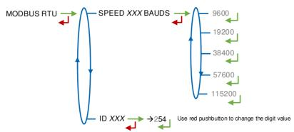
SPEED: Speed of the Modbus connection
