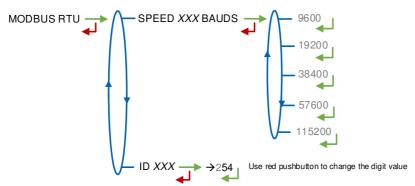
SPEED: Speed of the Modbus connection
