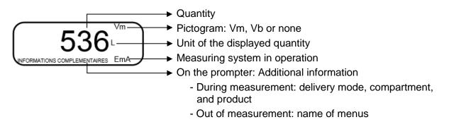
Configured data are pre-visualized thanks to menus. In the example above, XX corresponds to the value given to the conversion, either OFF or ON.
