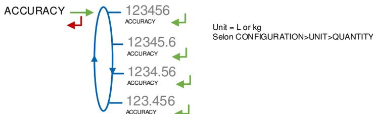
**FLOWRATE:** Choose the accuracy of the quantity that will be displayed and printed. According to the unit set in menu CONFIGURATION>UNIT>QUANTITY (measure of a volume or a mass).
