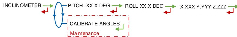
**PITCH...:** Used to display the bank angles of the truck and the inclinometer raw data
