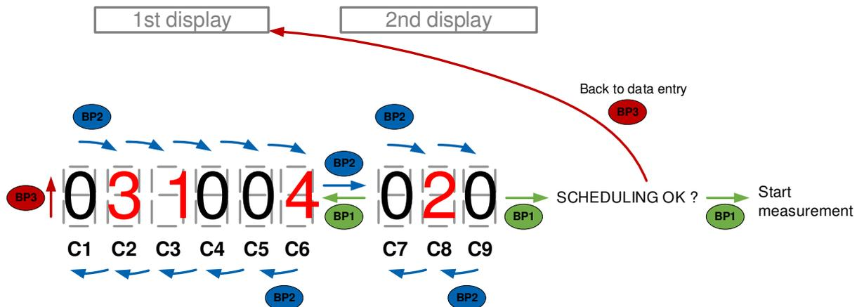
To include a compartment into the delivery, move on to the digit related to the compartment with BP1 (to the right) or BP2 (to the left), then validate with BP3. When you validate, the value 0 becomes the order number. When you validate again with BP3, the compartment is removed from the delivery, then the order numbers of the previous compartments are all decremented by one.
