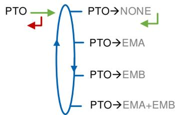
When the system operates with power take-off, select the relevant pumped measuring system (EMA, EMB or both). Then choose the transmission the truck is equipped with. It is used to take into account the engine start and stop, clutching and power take off.
