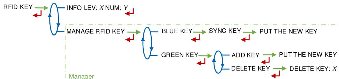
**INFO:** Display of the level and the identifier of the RFID key (blue key: Level1-User, green key: Level2-Manager, red key: Level3-Maintenance)
