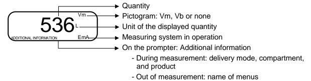
Configured data are pre-visualized thanks to menus. In the example above, XX corresponds to the value given to the conversion, either OFF or ON.
