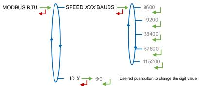
SPEED: Speed of the Modbus connection
