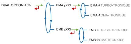
The system operates with two measuring systems EMA and EMB. For both one, configure the distribution ways.
