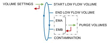
**START LOW FLOW VOLUME or START LOW FLOW MASS**: Volume or mass delivered in low flowrate before switching in high flowrate.
