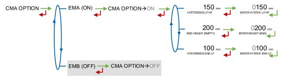
**HYSTERESIS LF-HF**: At the beginning of a measurement or following an intermediate stop. Before switching again from low to high flowrate, the calculator-indicator checks the total between LOW FLOW HEIGHT and HYSTERIS LF-HF.
