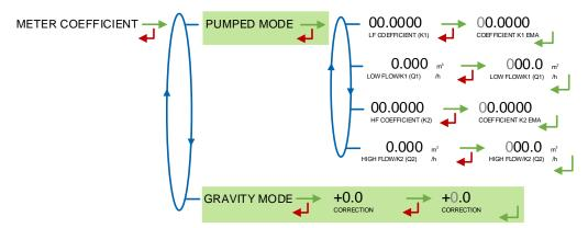
GRAVI-TRONIQUE PUMPED MODE: For pumped distribution mode, set the four items that follows
