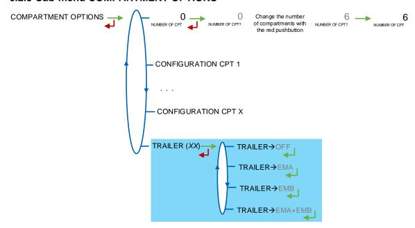
This menu is used to configure the compartments and their assignment to each measuring system, if required. First, set the number of compartments.
