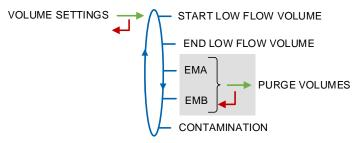
**START LOW FLOW VOLUME or START LOW FLOW MASS**: Volume or mass delivered in low flowrate before switching in high flowrate.
