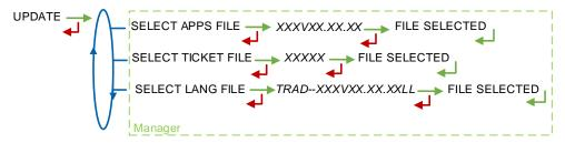
**SELECT APPS FILE (\*)** – Access restricted to the Manager with green key and/or to the Maintenance with red key. Used to display and select the version(s) of the application available on the SD card. NO FILE is displayed if there is no file to download.
