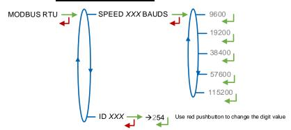
SPEED: Speed of the Modbus connection
