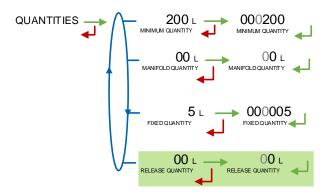
**MINIMUM QUANTITY**: Set the minimum quantity of the EMA measuring system. This value is given by the association of the turbine meter, the MICROCOMPT+ and other parts of the measuring system.
