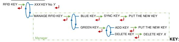
Displays the color and the identifier of the RFID key placed on the screen. E.g.: RED KEY No 123 **MANAGE RFID KEY** – *Access restricted to the Manager*:
