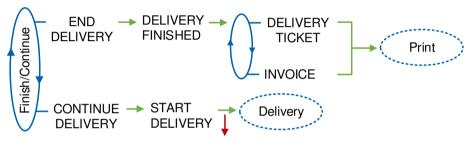
You can change the criteria: press the red pushbutton when START DELIVERY is displayed with the volume already discharged.
