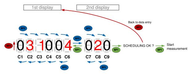
To include a compartment into the delivery, move on to the digit related to the compartment with BP1 (to the right) or BP2 (to the left), then validate with BP3. When you validate, the value 0 becomes the order number. When you validate again with BP3, the compartment is removed from the delivery, then the order numbers of the previous compartments are all decremented by one.
