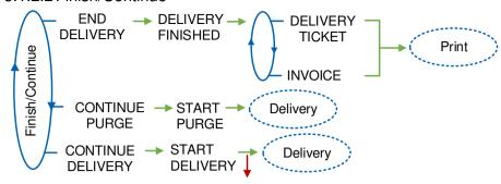
You can change the criteria: press the red pushbutton when START DELIVERY is displayed with the volume already discharged.
