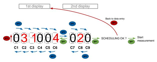
To include a compartment into the delivery, move on to the digit related to the compartment with BP1 (to the right) or BP2 (to the left), then validate with BP3. When you validate, the value 0 becomes the order number. When you validate again with BP3, the compartment is removed from the delivery, then the order numbers of the previous compartments are all decremented by one.
