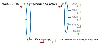
SPEED: Speed of the Modbus connection
