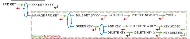
**KEY**: Displays the color and the identifier of the RFID key placed on the screen. E.g.: RED KEY (0123)
