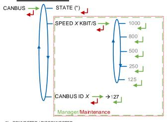
(\*) CONNECTED / DISCONNECTED (\*\*) BETWEEN 1 AND 127
