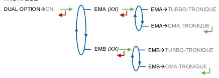
The system operates with two measuring systems EMA and EMB. For both one, configure the distribution ways.
