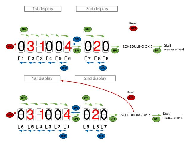
To include a compartment into the delivery, move on to the digit related to the compartment with BP1 (to the right) or BP2 (to the left), then validate with BP3. When you validate, the value 0 becomes the order number. When you validate again with BP3, the compartment is removed from the delivery, then the order numbers of the previous compartments are all decremented by one.
