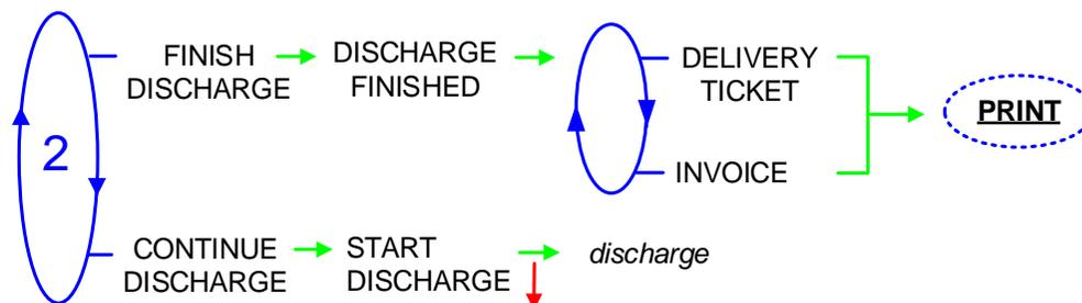
**To change the delivery mode:** press the red pushbutton when "START DISCHARGE" is displayed with the volume already discharged.
