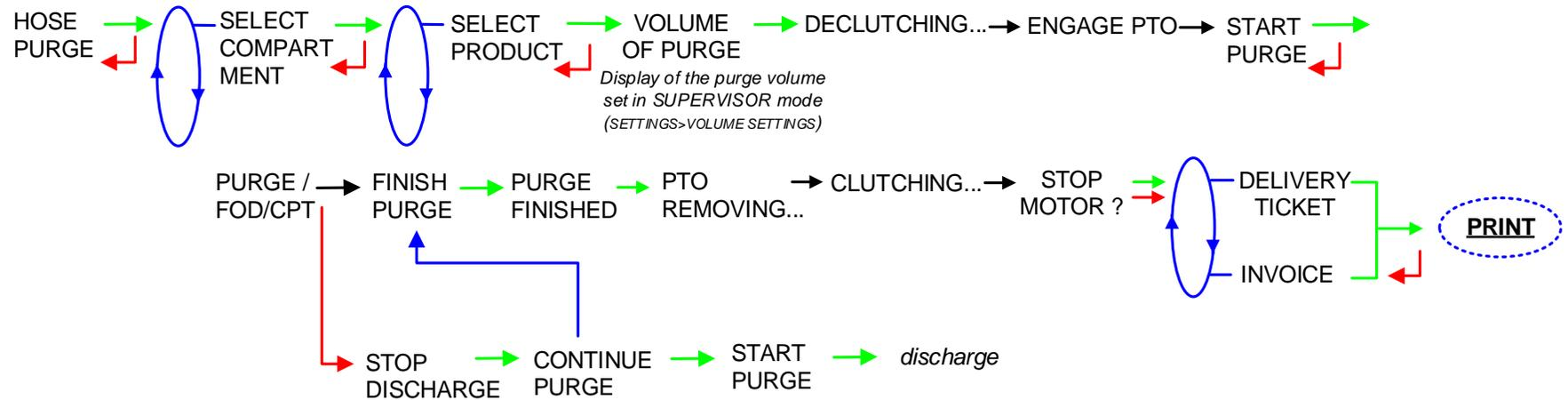
4.3.1.6 With Compartment selection + Return valve + Motor control (PTO)
