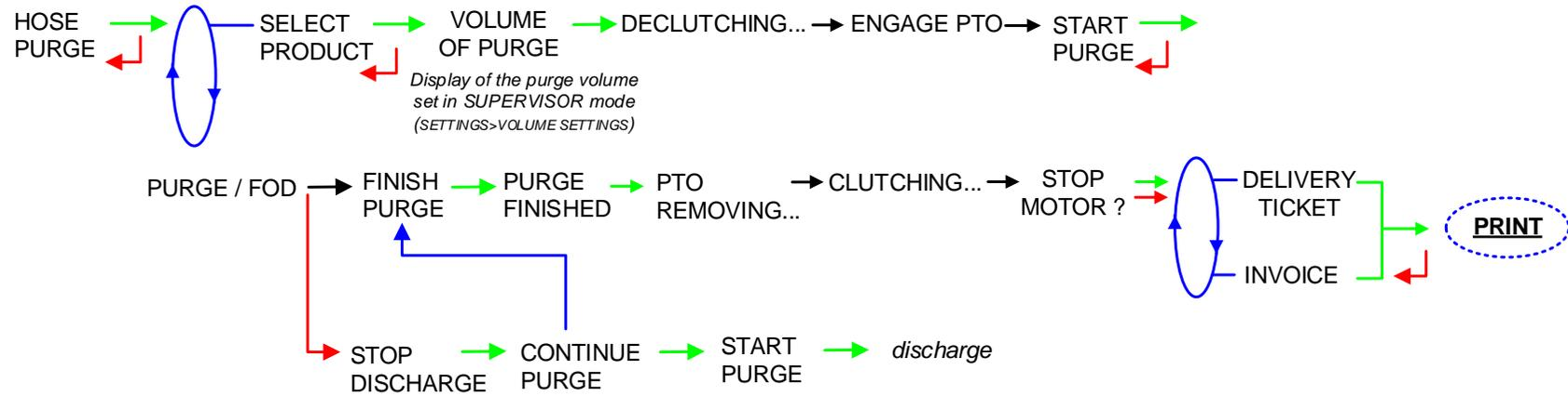
4.3.1.5 With Compartment selection + Motor control (PTO)
