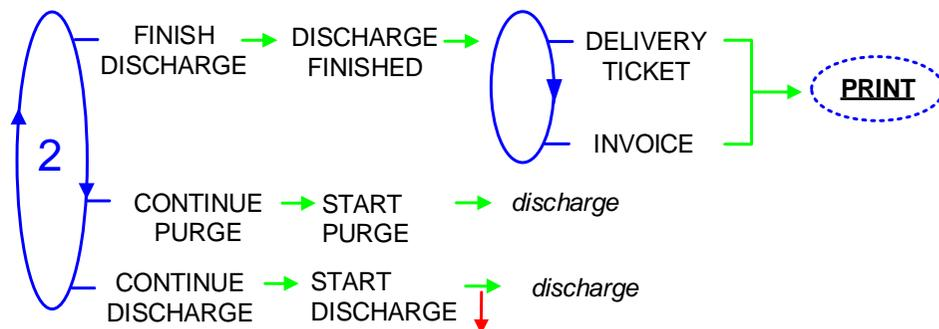
***To change the delivery mode:*** press the red pushbutton when "START DISCHARGE" is displayed with the volume already discharged.
