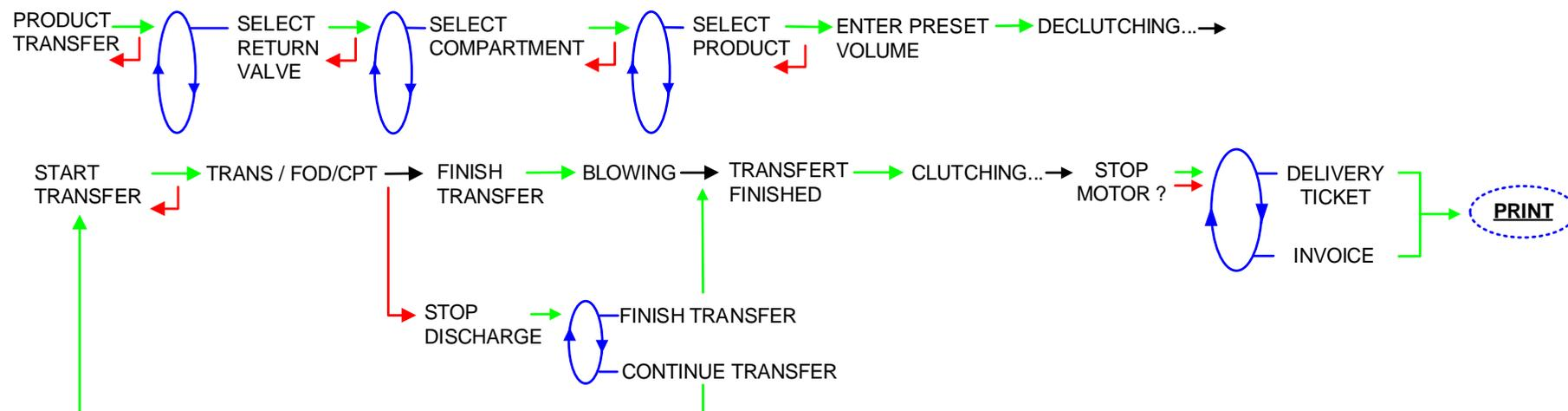
4.3.2.2 A With Compartment selection + Return valve + Motor control (PTO)
