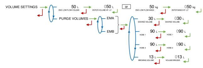
**END LOW FLOW VOLUME or END LOW FLOW MASS**: Volume or mass delivered in low flowrate to finish the delivery
