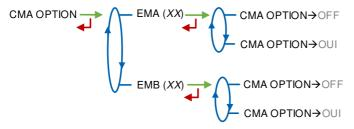
For each CMA TRONIQUE measuring system, the menu gives access to the configuration of specific parameters:
