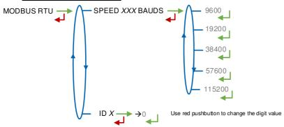
**SPEED**: Speed of the Modbus connection
