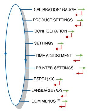
**ICOM MENUS** <sup>(1)</sup>: The sub-menus are different according to the level of access: Level1-User, Level2-Manager and Level3-Maintenance.
