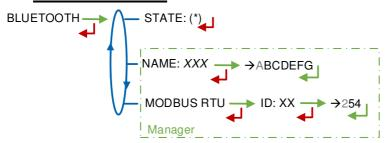
(\*) NOT AVAILABLE (the calculator is not equipped) / DISCONNECTED / CONNECTED
