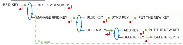
**INFO**: Display of the level and the identifier of the RFID key (blue key: Level1-User, green key: Level2-Manager, red key: Level3-Maintenance)
