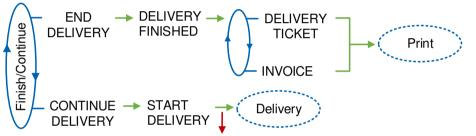
You can change the criteria: press the red pushbutton when START DELIVERY is displayed with the volume already discharged.
