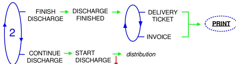
**To change the delivery mode:** press the red pushbutton when "START DISCHARGE" is displayed with the volume already discharged.
