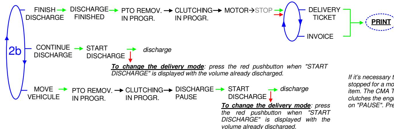
If it's necessary to move the vehicle, the distribution has to be stopped for a moment, then choose the "MOVE VEHICLE" item. The CMA TRONIQUE switches off the power take-off, clutches the engine and freezes the MICROCOMP indicator on "PAUSE". Press green button to continue distribution.
