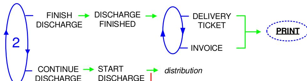
**To change the delivery mode:** press the red pushbutton when "START DISCHARGE" is displayed with the volume already discharged.
