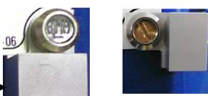
Sealed cup protecting access to metrological functions
