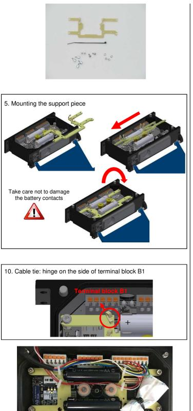
The support piece is used to lock the batteries and to make sure the wires or the packet don't get caught when closing the UNI-2.
