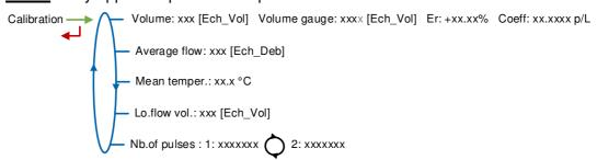
**Volume**: Display the volume; **Gauge volume**: Enter the volume read on the calibration mean; **Er**: Display the error in %; **Coeff**: Coefficient to be set only by an authorized person in METROLOGICAL mode, if required
