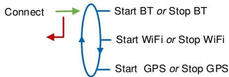
**Start BT:** Start or stop Bluetooth connection. The Bluetooth switches automatically to stand-by mode after two minutes of inactivity when connection is off and after ten minutes of inactivity when connection is on
