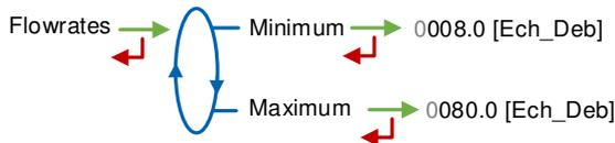
**Minimum:** Minimum flowrate of the measuring system. Unit depends on the configuration (Config.>Scales>Flowrates)
