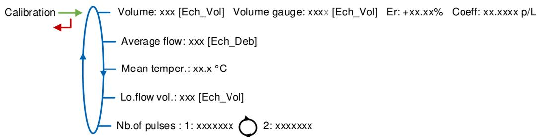
**Volume:** Display the volume; **Gauge volume:** Enter the volume read on the calibration mean; **Er:** Display the error in %; **Coeff:** Coefficient to be set only by an authorized person in METROLOGICAL mode, if required
