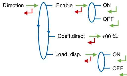
**Enable:** Choose ON if the UNI-2 is intended to detect the loading direction and is able to sum loading volumes in a specific totalizer (non guaranteed volumes)
