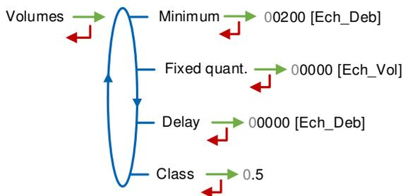
**Minimum:** Minimum measured quantity to guaranty the measurement. Unit depends on the choice made for the scale interval
