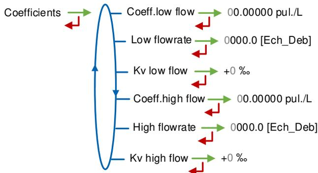
When parameters **Low flowrate** and **High flowrate** are set to zero, parameters **Coeff.high flow** and **Kv high flow** are not applied.
