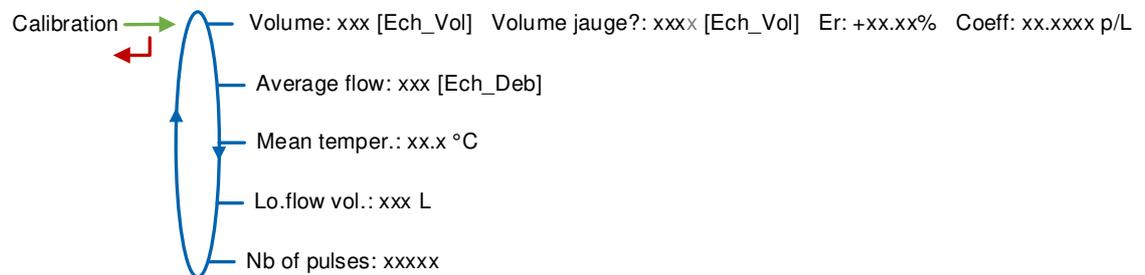
**Volume:** Display the volume; **Gauge volume:** Enter the volume read on the calibration mean; **Er:** Display the error in %; **Coeff:** Coefficient to be set only by an authorized person in METROLOGICAL mode, if required
