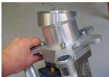
*Positioning upstream bent sleeve*
