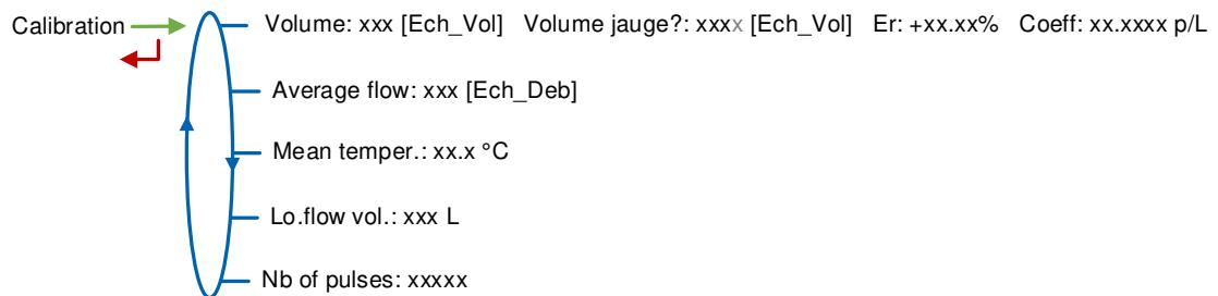
**Volume:** Display the volume; **Gauge volume:** Enter the volume read on the calibration mean; **Er:** Display the error in %; **Coeff:** Coefficient to be set only by an authorized person in METROLOGICAL mode, if required
