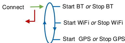
**Start BT:** Start or stop Bluetooth connection. The Bluetooth switches automatically to stand-by mode after two minutes of inactivity when connection is off and after ten minutes of inactivity when connection is on
