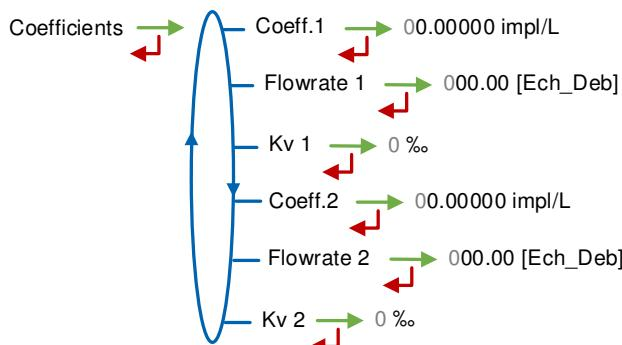
When parameters Flowrate 1 and Flowrate 2 are set to zero, parameters Coeff.2 and Kv 2 are not applied.
