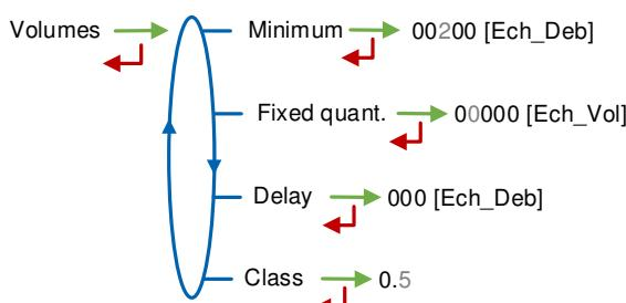
**Minimum:** Minimum measured quantity to guaranty the measurement. Unit depends on the choice made for the scale interval
