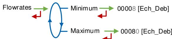
**Minimum:** Minimum flowrate of the FLEXICOMPT AUTONOME+. Unit depends on the configuration (Config.>Scales>Flowrates)
