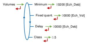
**Minimum**: Minimum measured quantity to guaranty the measurement. Unit depends on the choice made for the scale interval
