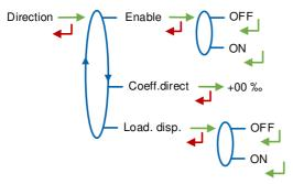
**Enable**: Choose ON if the UNI-2 is intended to detect the loading direction and is able to sum loading volumes in a specific totalizer (non guaranteed volumes)
