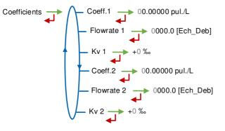
When parameters Flowrate 1 and Flowrate 2 are set to zero, parameters Coeff.2 and Kv 2 are not applied.
