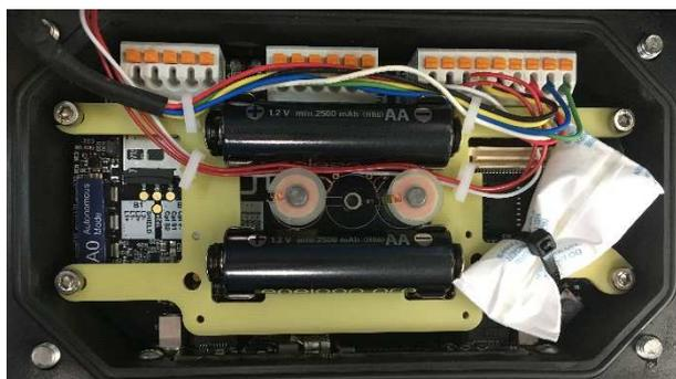
The support piece is used to lock the batteries and to make sure the wires or the packet don't get caught when closing the UNI-2.
