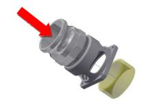
Remove the sight glass with the screwdriver or with the pin punch and the hammer
