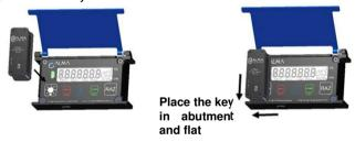
Press simultaneously RAZ and Select for at least 2 seconds
