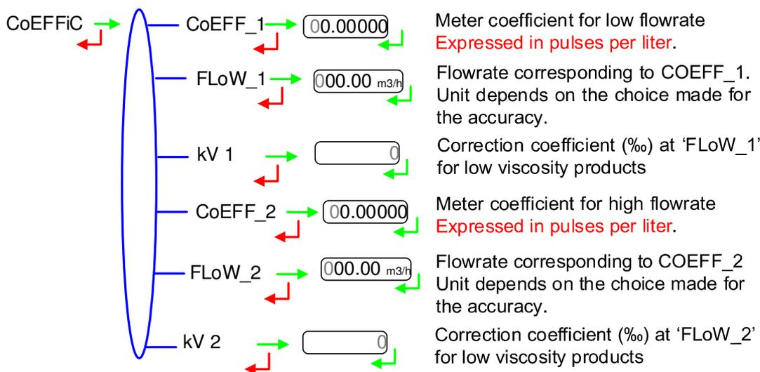
When parameters FLoW\_1 and FLoW\_2 are set to zero, parameters CoEFF\_2 and kV 2 are not applied.
