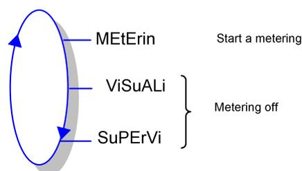
The UNI metering can be either ON or OFF. Metering is ON between the first command level after initialisation or resetting the current volume to zero, and resetting the current volume to zero.
