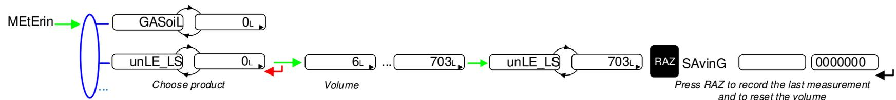
If data recording is automatic, the time required at the end of measurement before recording must be set in METROLOGICAL mode (menu 'Aut SAV').
