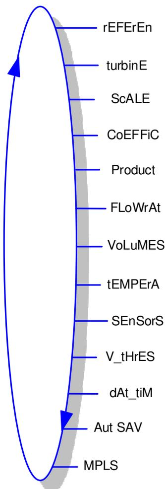
The configuration parameters can only be modified after the processor configuration switch on the electronic card has been switched over. Only authorized personnel can modify these parameters.
