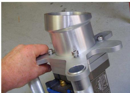
*Positioning upstream bent sleeve*
