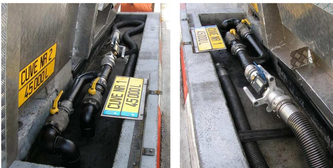
Examples of improper stationary installation of the FLEXICOMPT AUTONOME+:
