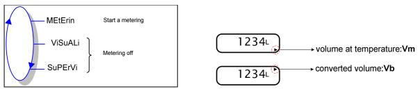
The UNI metering can be either on or off. Metering is ON between the first command level after initialisation or resetting the current volume to zero, and resetting the current volume to zero.
