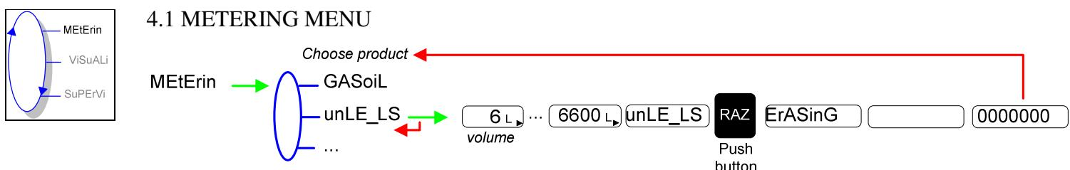
Use BP2 to display flow rate (and temperature) during measuring.
