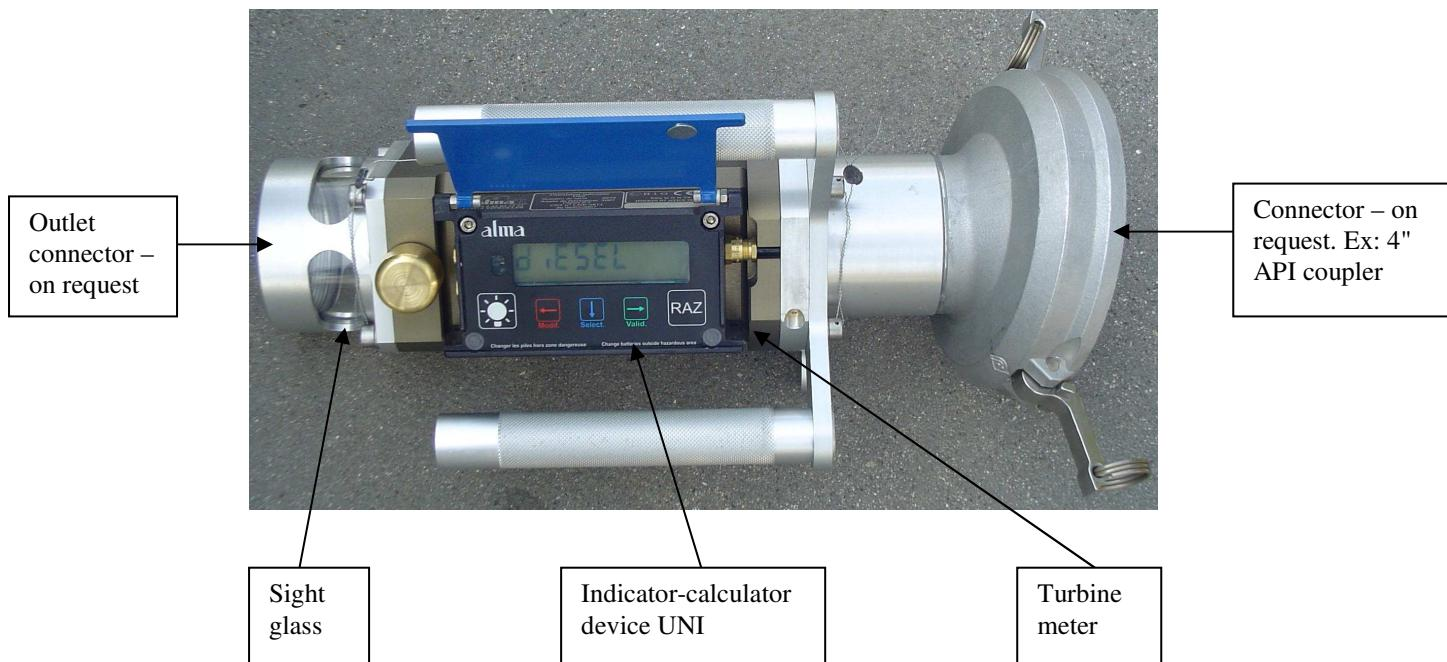
The indicator-calculator device, type UNI guarantees the metering operation and manages the faults linked with the metering system.
