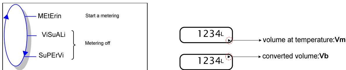
The UNI metering can be either on or off. Metering is ON between the first command level after initialisation or resetting the current volume to zero, and resetting the current volume to zero.
